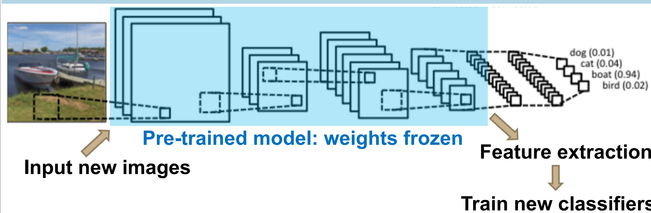
Fig.2. To reuse a pre-trained CNN model that has been trained by image datasets from other fields (WildML, 2015)
